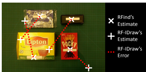
Figure 9: Sample output of the estimated RFID locations by RFind and RFIDraw. RFind’s location estimations (indicated by crosses) enable pinpointing the location of the items they tag whereas RFIDraw’s estimations (indicated by x’s) cannot assign an RFID’s location to the item it tags.
