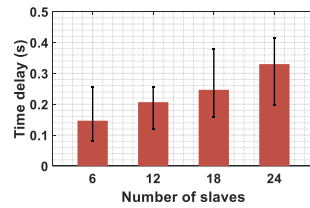
Figure 18: Beamforming delay vs. number of slave radios.
